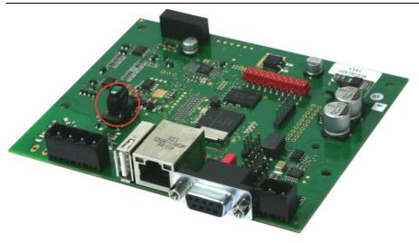
Figure 1 Location of the missing PLC Transformer
